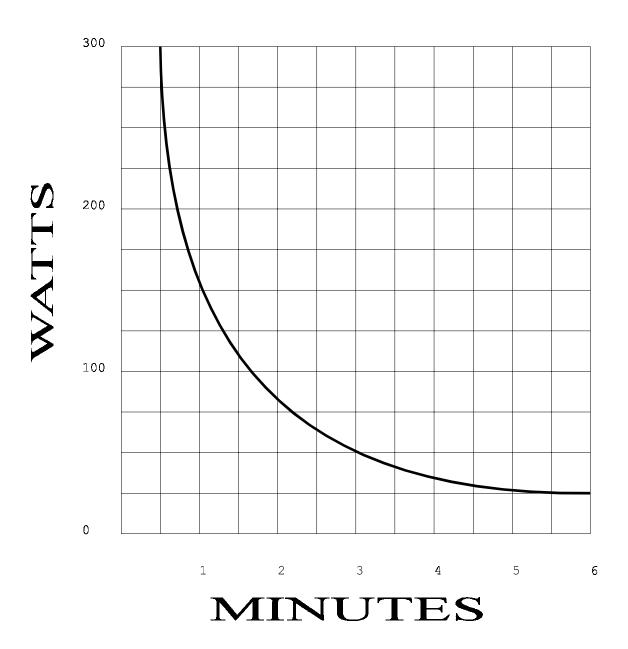
Derating curve for the MFJ260 Dummy Load.
